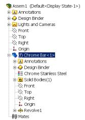
Mates may be used to fully define a component that does not move, or under define a component that is intended to move.
